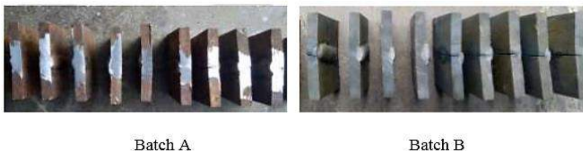
Figure 1: Mild steel welded samples
