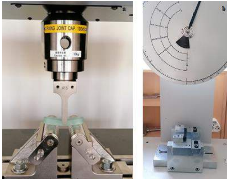
Figure 4. Three-point bending (a) and Charpy impact (b) tests
