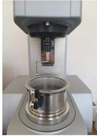
Figure 1. Rheometer, measuring cup and ball system used in the study
