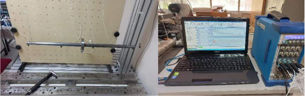
Figure 5. The experimental rotor system and one of the measurement of the modal test
