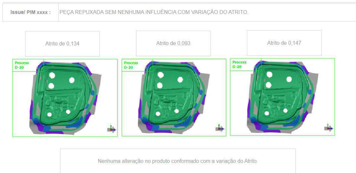
Figure 5 - Numeric Simulation - New Friction Coefficients
