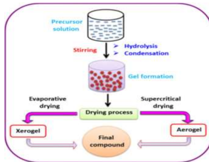
Figure 1. The stages of the sol-gel formation process.
