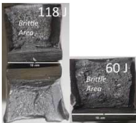
Figure 8. Fractured Charpy impact test specimens.
