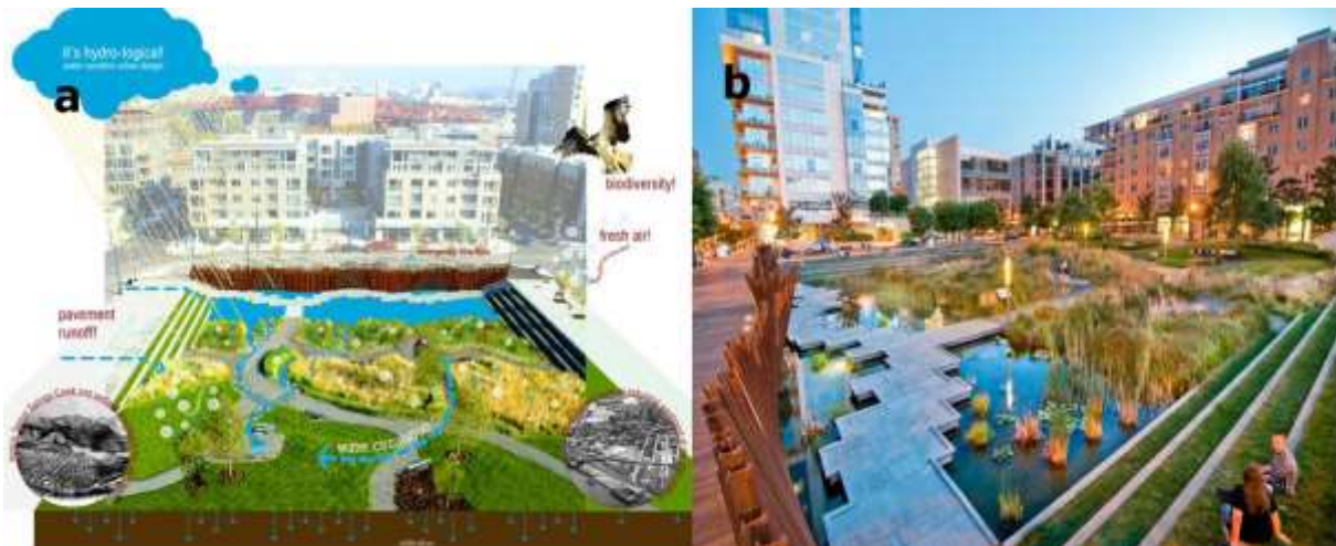
Figure 7. Tanner Springs Park's drainage system (a) and blue-green infrastructure application in the park (b) (Kruse, 2015).
