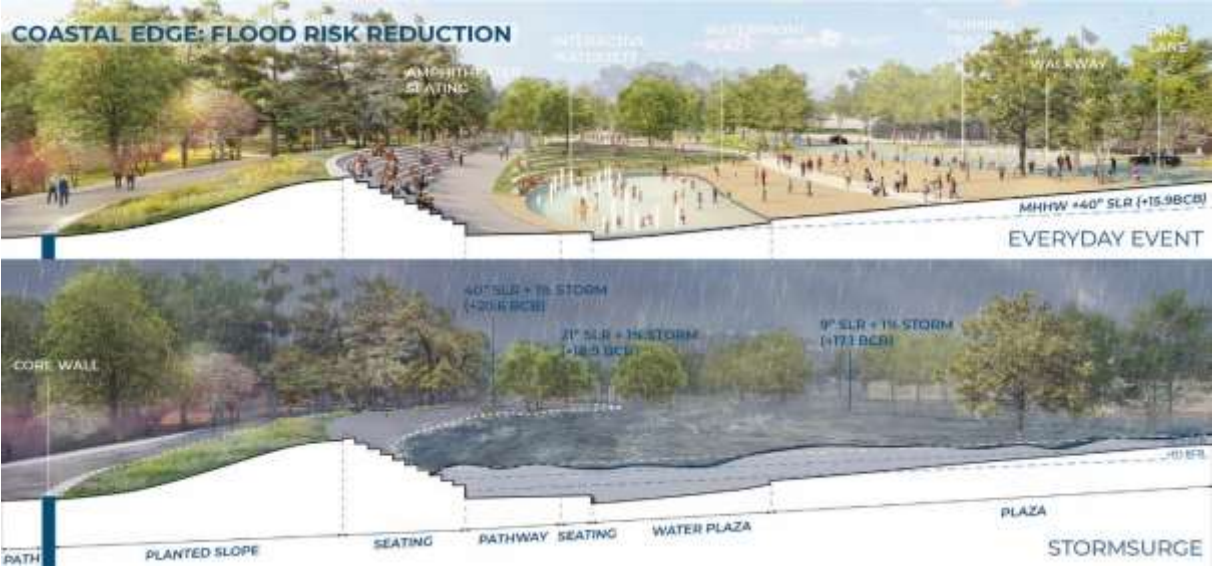
Figure 8. Moakley Park Resilience Plan-landscape design for coastal area flood risk reduction (ASLA, 2022).
