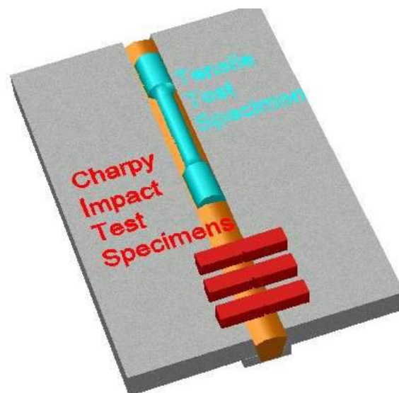
Figure 1. All weld metal design.
